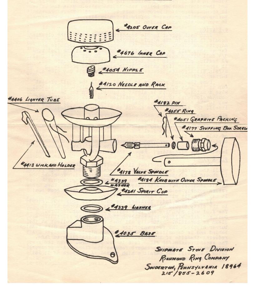
The kerosene burners in your Shipmate Kerosene Stove convert liquid kerosene into a vapor which is then burned. This is accomplished by passing the liquid kerosene up through hollow tubes in the burner to a hollow ring at the top of the burner and then down another hollow tube to the valve. When the valve is opened, vaporized kerosene must be released. Therefore the burner must be preheated before it can be lit. Once a burner is started the vaporization is automatic.
